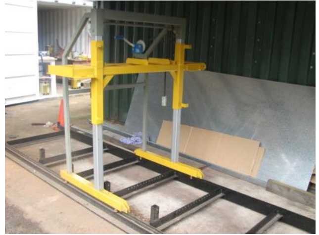
Work progresses steadily on the new Slabbing Saw.
