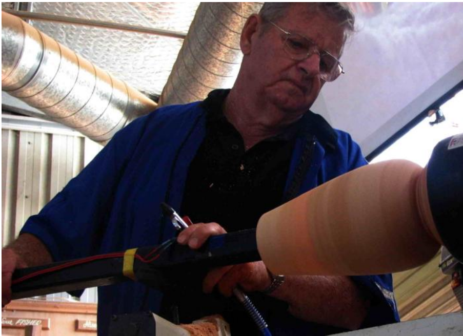
The light shows up any variations of thickness in the wall of the bowl.
