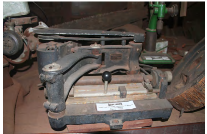
This is an old professional dovetail cutter. Has it's own "router" (an electric motor).
