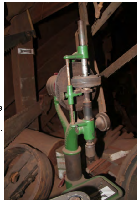
This is an old professional dovetail cutter. Has it's own "router" (an electric motor).
