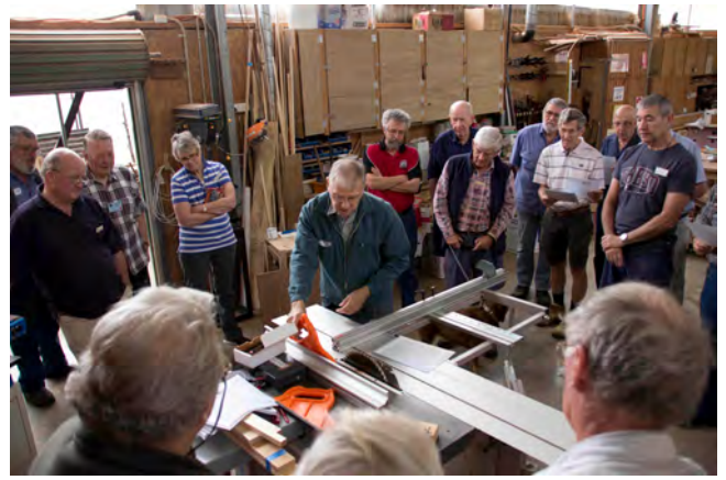
Last week a large group of Woodies were treated to a very enlightening demo by Rob Otto of the do's and dont's of using the Hammer table saw. Safety was the overriding feature of the demonstration as well as the use of Jigs to achieve repeated accurate results.
