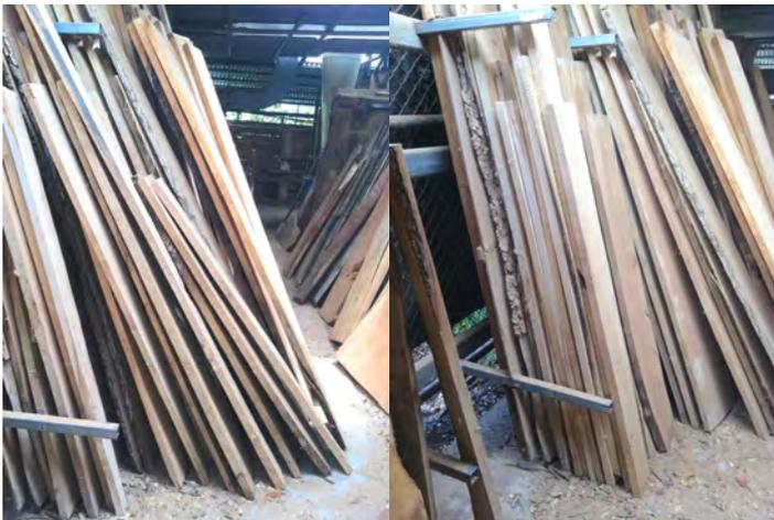
Inspect the photo on the left of a stack of timber in our Wood Shed and notice how each piece of timber is supported at two points....its top and bottom. This leaves the centre of the board unsupported and therefore subject to bending which makes it more difficult to process for use and also more waste.
