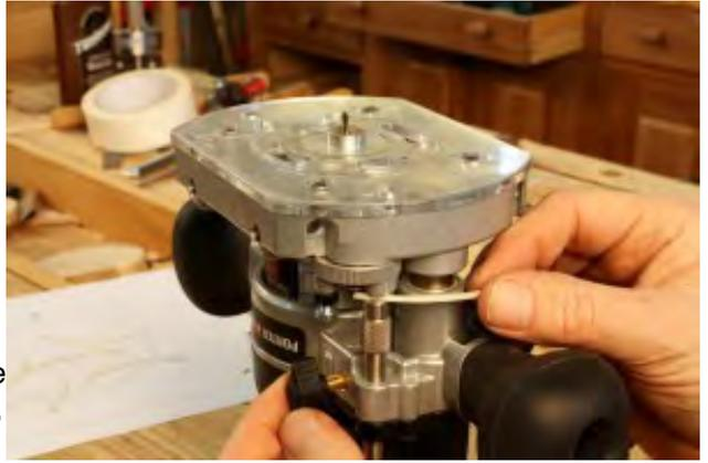
The trick is to set the depth to dead zero on a flat surface, tighten the depth control lever, then invert the router, release the depth stop rod, insert the piece of inlay between it and the stop and tighten the rod.
