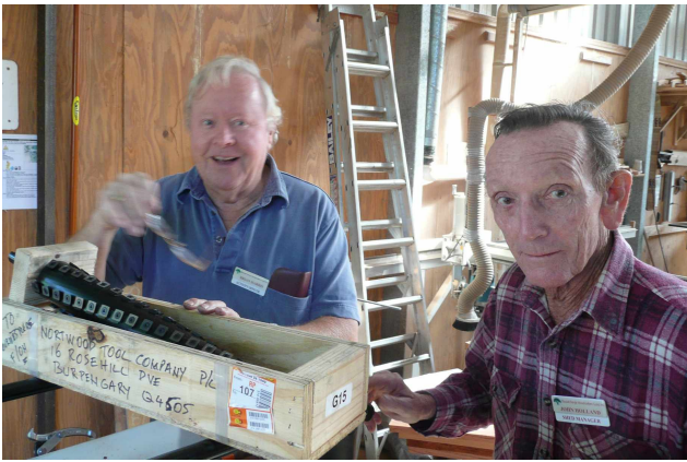
Brian Harris and John Holland unpacking the helix spiral cutter for the 15" thicknesser, prior to installation. The replacement was not a simple job, certainly not a case of plug and play. However, the results are said to be very smooth and very quiet.
