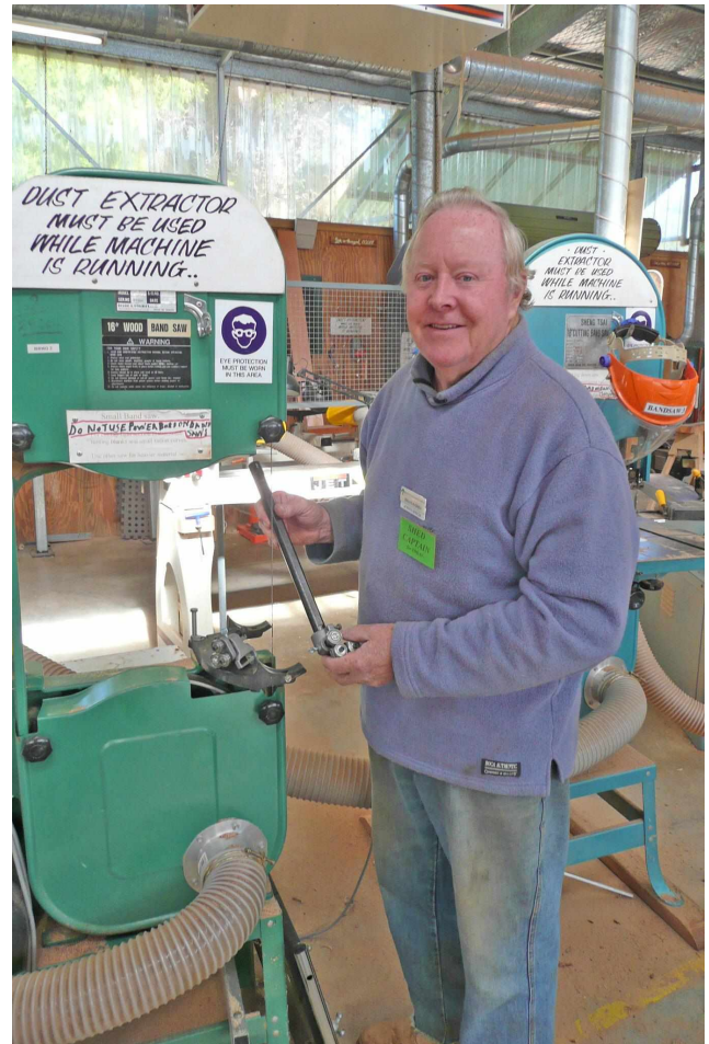
Brian Harris fixing the guide on Bandsaw #2. The new guide rollers will provide a much better operation.
