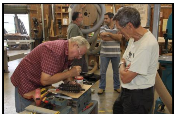
Brian replacing the cutters on the jointer
