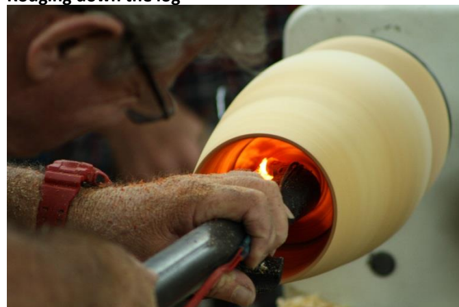
The brilliant use of light to gauge wall thickness
