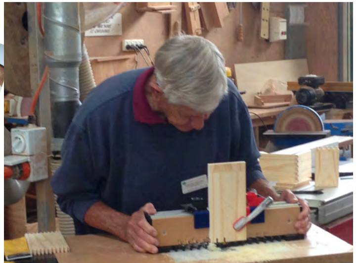
Lionel Tilley demonstrated the way to make perfect dovetails using the Gifkin Jig.
