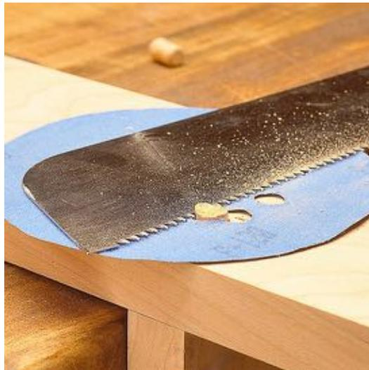
A disc placed abrasive-side down around the plug prevents minor saw tooth scratches should you accidentally pivot the blade.
