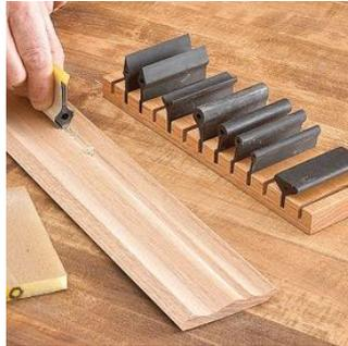
Foam sanding pads work well on broad curves, but contour sanding grips reach into and around tight curves and V-grooves.
