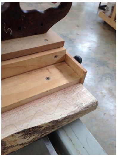
The end of the jig can be adjusted to determine the width of the piece of wood you wish to cut.
