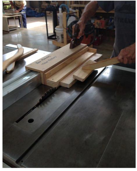
If there is a need to cut a narrow or several narrow timber strips of the same thickness there are a number of ways of doing this. Recently the manufacture of a shop built jig at our club will allow for the safe cutting of such strips with no possible risk for damage to the fence. For instruction on how to use this jig please see Phil Lane.
