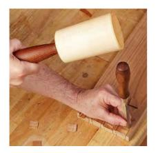
A wood mallet with a large head requires less precision when striking a chisel, so you can concentrate on making the cut.
