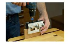
Drill the magnet hole in the leg using a self-centring dowel hole drilling jig and a 1/4" dia. drill bit. Set the bit depth to 7/16" which will make the magnet hole 1/8" deep once the notch is cut. Err on the hole being too shallow now since you can always make it deeper later. Too deep now will mean you have to somehow fill the excess depth later.
