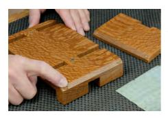
The final step is to add rubber door bumpers to the beveled ends of the leg and platform. These bumpers keep the stand from sliding when it's set up in either the high or the low position.
