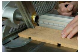
Using your miter gauge and stop again, cut the beveled ends using a fine-cut cross-cut saw blade. The saw blade is set to 45-degrees.
