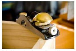
Block planes have become one of the most oft-used tools in a woodworker's workshop. Some traditional woodworkers even keep them in their aprons! These little planes can be used to trim your joints, put chamfers on board edges, trim end grain, etc.
