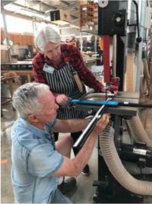
Colleen using the jig to cut circles on the bandsaw - with Kev Devlin's guidance
