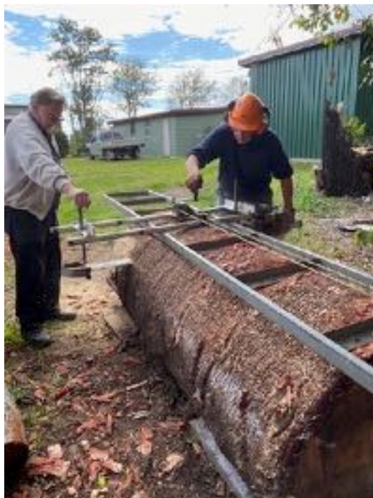
The millers using the the chain saw mill to get a Bunya pine log down to a size they could put through the mill.
