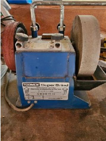
Tormek Super Grind wet grinder complete with various sharpening jigs.
