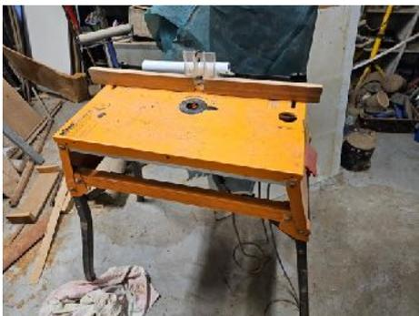
Triton router table with 1/2" Makita router (Best router made by Makita.)
